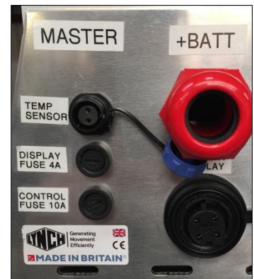
Temperature sensor socket on controller
