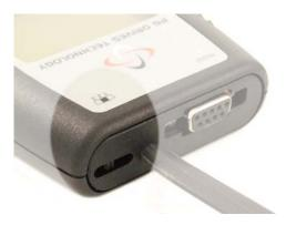
For normal Sigmadrive programming and diagnostics, this switch must be set to position 2.
