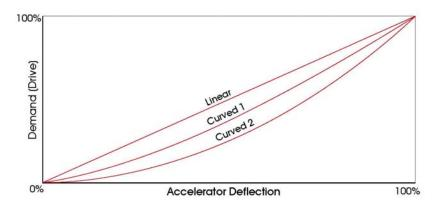
This sets the type of response for both the Accelerator and Footbrake inputs (pins 8 & 9 on Connector A). There are three options for Permanent Magnet Traction control, Linear, Curved1 and Curved2.
