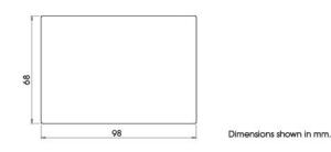
Before cutting the hole, ensure that enough room is available within the dash for the area of the module and the Securing Bracket. Access to the back of the dash will be required to secure the Sigmagauge.
