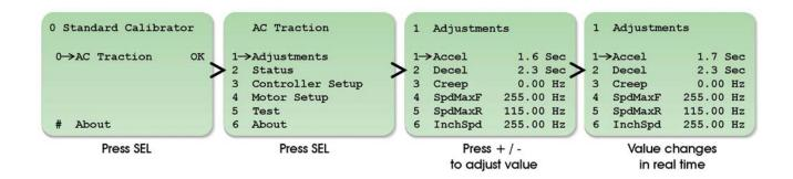
Some parameters e.g. 3.8 Truck Type Select, require that the power to the controller be cycled via the keyswitch before the new value will be accepted. These parameters are marked on the Programmer's screen with the word 'Key'.
